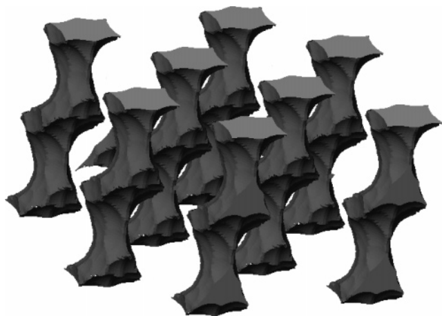
Figure 15. Representation of channels along the c -axis in the network resulting from crystallization of tecton 7 from DMSO/dioxane. The image shows a 2 \times 2 array of unit cells. The outsides of the channels appear in dark gray, and light gray is used to show where the channels are cut by the boundaries of the array. The surface of the channels is defined by the possible loci of the center of a sphere of diameter 6 Å as it rolls over the surface of the ordered network. 36
